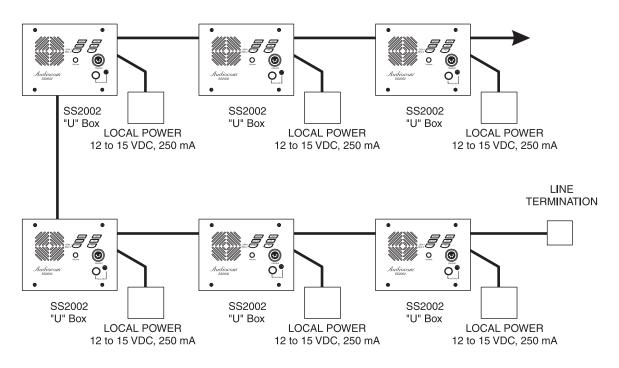
Figure 7 - An example of an Audicom intercom system using all locally powered "U" box stations, with no power being distributed on the intercom channels (dry lines). Since an Audiocom power supply is not used, the installer must connect a line termination somewhere in each channel for proper operation.
